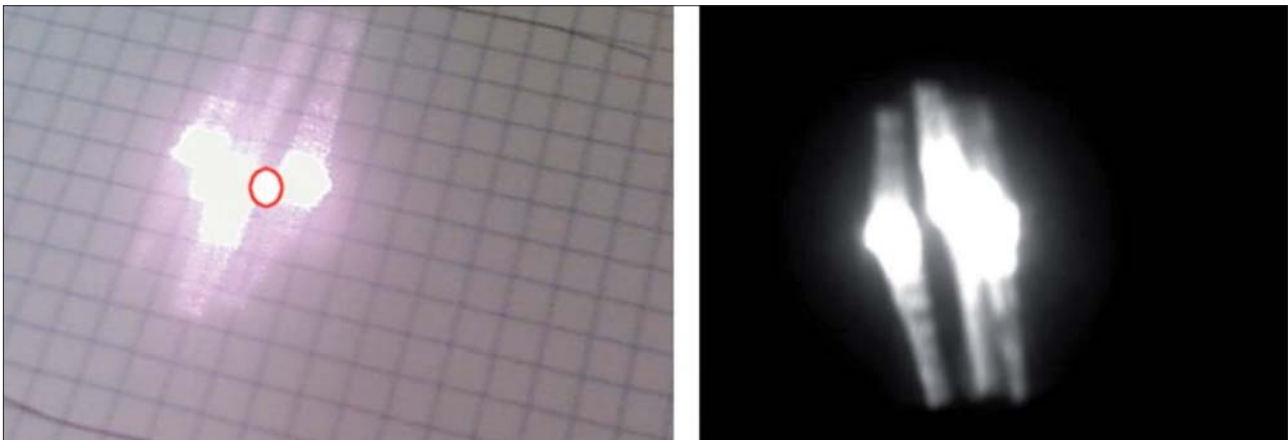
Figure 2. a) aiming beam (in the circle) and treatment beam are aligned but the treatment spot is not uniform, b) same laser spot captured by an IR camera
