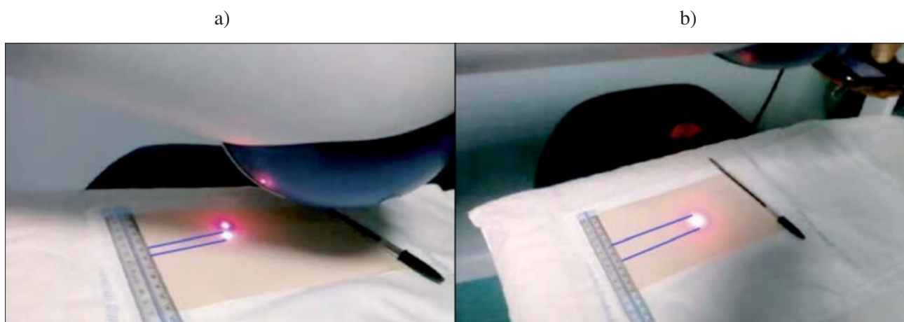
Figure 1. Treatment beam and alignment beam for laser 2, at 3 cm a) and at 38 cm b); the blue lines have been traced to evaluate spot diameter
