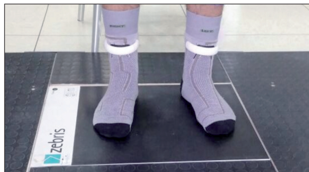
Figure 3. Test subject standing on the zebris® pressure plate while wearing Sensoria Socks
